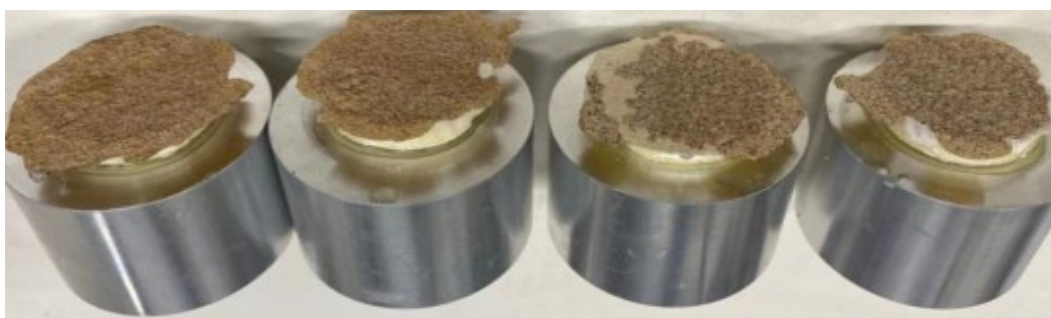
Adhesion testing showing substrate failure
