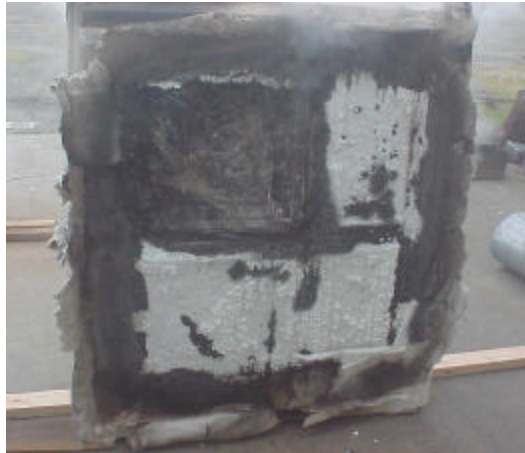
Figure 9. Post Test -- Exposed Face, Cracked Gypsum Board
