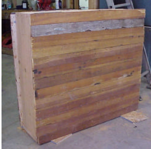
Figure 4. T & G Flooring as Assembly Unexposed Face
