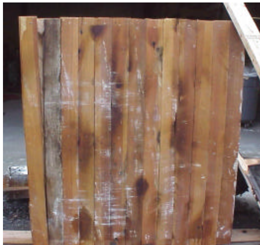
Figure 10. Post Test -- Unexposed Face Floor Finishing
